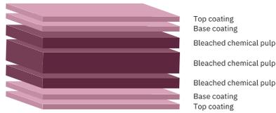
Invercote is a multi-layered product (solid bleached board, SBB), entirely based on fresh fibres. Specific fibre compositions are used for the various layers in the construction to optimise performance. The outer layers are dominated by hardwood fibres to promote smoothness and printability. The middle layer consists of softwood fibres for strength and flexibility.
